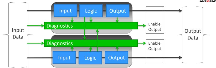
If an ECU fails in one of the two channels, the system does not shut down but continues to operate with only one channel **The best policy is not to operate on a single channel for a "long" period of time.**
